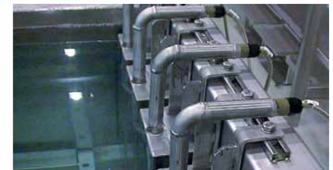
Ultrasonic components add power to existing cleaning systems.
