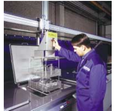
Pneumatically operated assisted lift for easy basket handling. Loads up to 50 kg.
