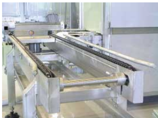
Motorised chain conveyor for loading and unloading provides storage buffer. Gravity conveyor for light weights.
